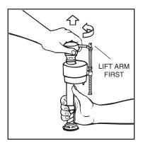
IMPORTANT: Always clear sand and rust from system. Make sure water supply is off. Remove valve TOP by lifting arm and rotating top and arm 1/8 turn counterclockwise, pressing down slightly on cap.
